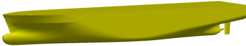
**Fig. 1 Geometry model of KCS (Case 2.10)**
