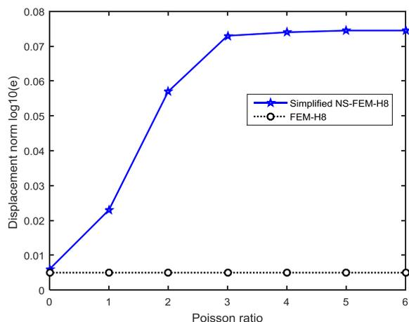
Figure 6 Displacement norm versus different Poisson's ratios for the hollow sphere subjected to inner pressure.
