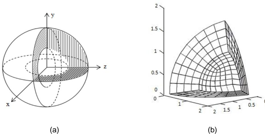
Figure 3 (a) hollow sphere problem domain and (b) one-eighth model discretized using eight-noded hexahedron elements.
