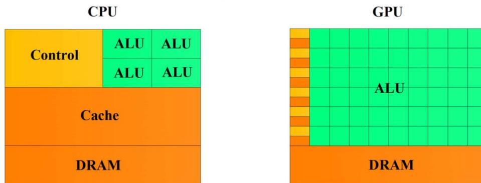
**Figure 1. Different hardware architectures for GPU and CPU**
