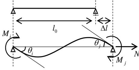
**Fig.1 Element edge force and beam deformation in small deformation theory**
