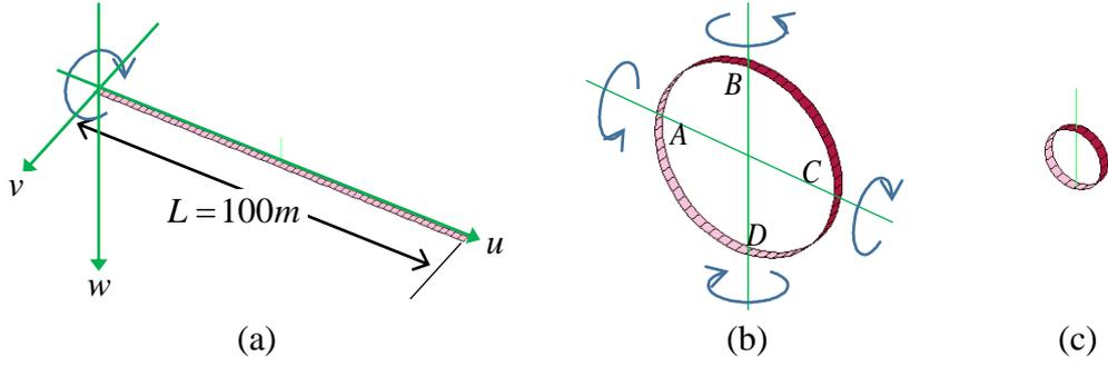
$E = 210GPa, G = 81GPa$ , Cross section:  $1m \times 0.05m$  of rectangle
