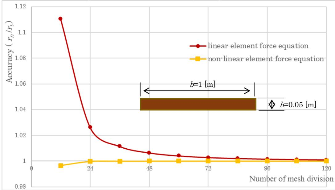
**Fig.4 Accuracy of numerical solutions (Section aspect ratio:20)**
