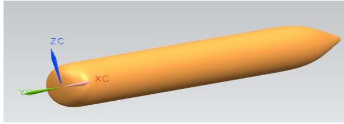
**Figure 1. Bare body shape of NWPU PAUV**
