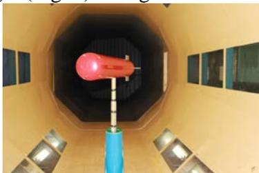
**Figure 5. Side slip angle change test**
