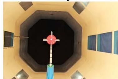
**Figure 6. Elevators deflection angle change test**
