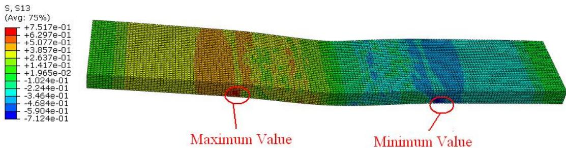
Fig.5 Stress (S13) contour of foam core
