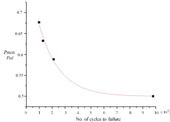
Fig.3 Modified S-N curve data for foam core sandwich structure on fatigue life
