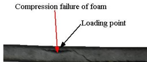
Fig.2 Failure modes of foam core sandwich beams
