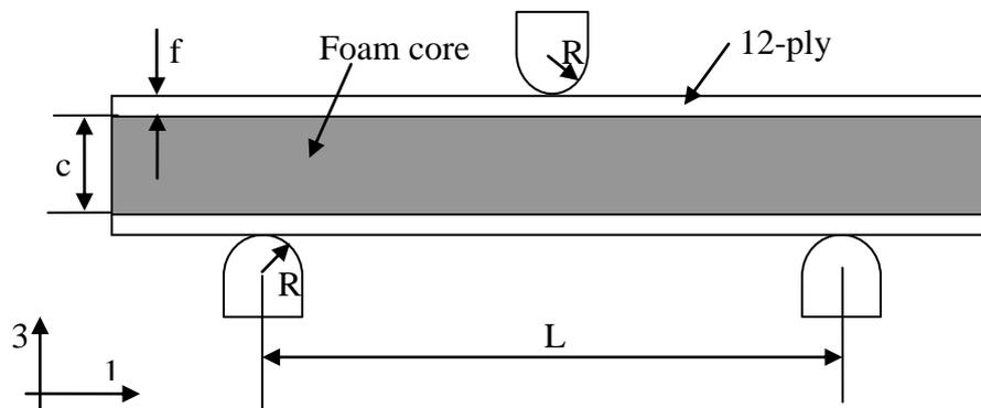
Fig.1 Three-point bending of sandwich beam with indenter and supports
