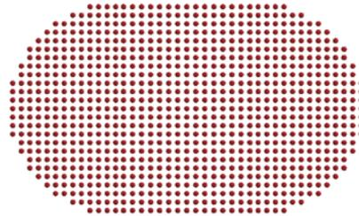
(b) SPH bird model with 16041 particles
