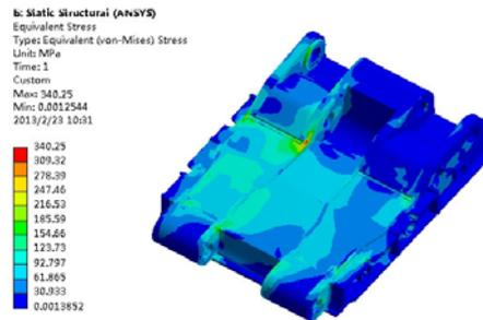
**Figure 5. Optimized stress distribution of the shield beam**
