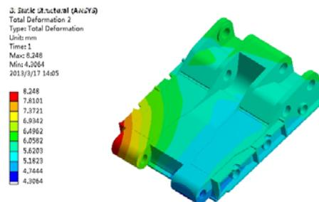
**Figure 6. Optimized deformation of the shield beam**
