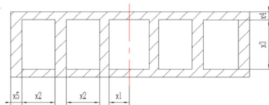
Figure 4. The shield beam's cross section
