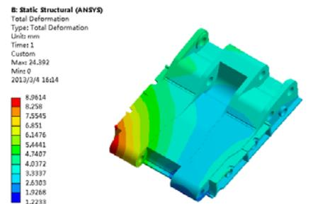
Figure 2. Shield beam's deformation
