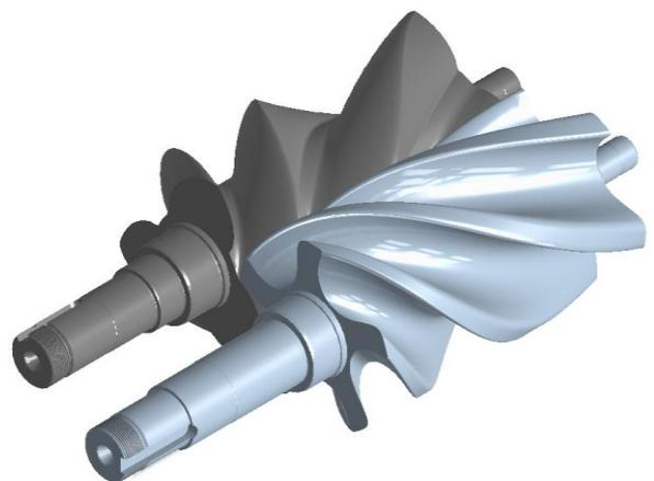
**Figure 2.** Variable Pitch Screw Rotors
