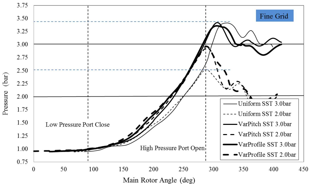
**Figure 10. Indicator diagram**
