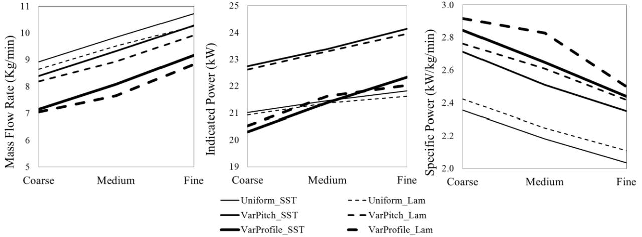
**Figure 11. Effect of grid refinement on integral parameters**
