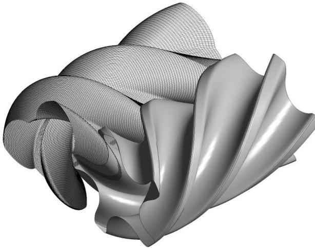
**Figure 6. Numerical grid for variable pitch screw rotors**
