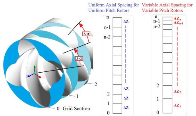
Figure 4. Cross sectional spacing for uniform and variable pitch rotors
