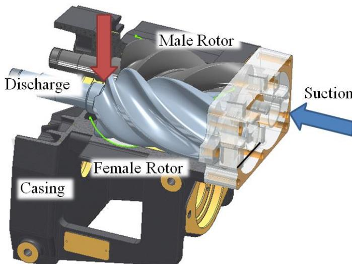
**Figure 1.**Sectioned view of a Twin Screw Compressor
