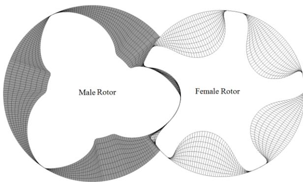
Figure 3. Numerical grid in a cross section
