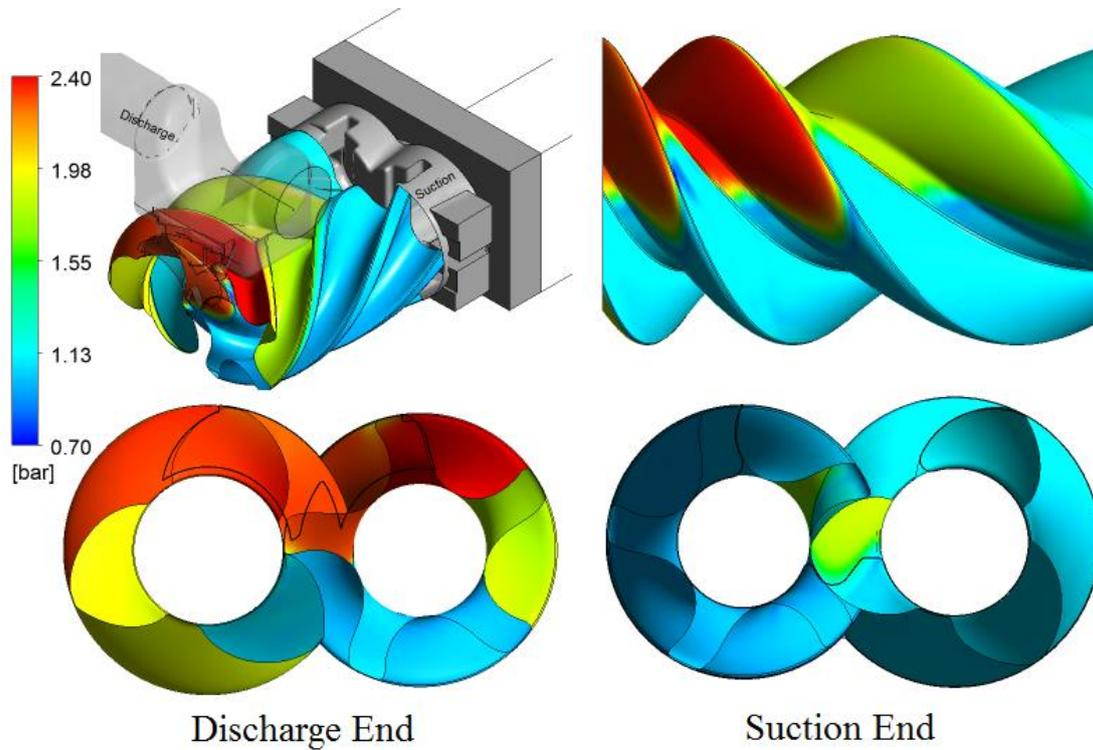
**Figure 9. Pressure variations in the variable pitch rotors with discharge pressure 2.0 bar**
