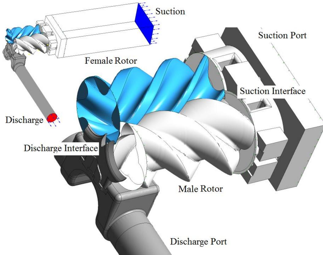
**Figure 8. Compressor model with variable profile rotors**
