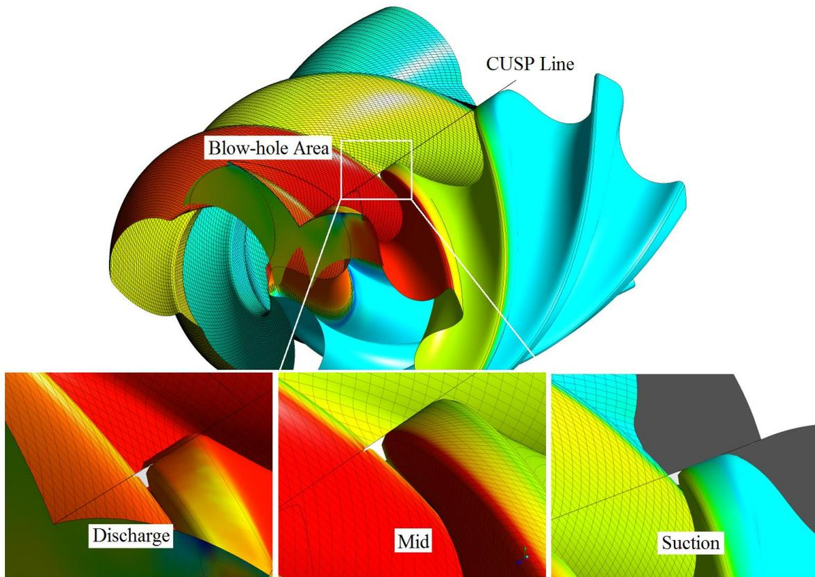
**Figure 13. Comparison of Blow-hole area**
