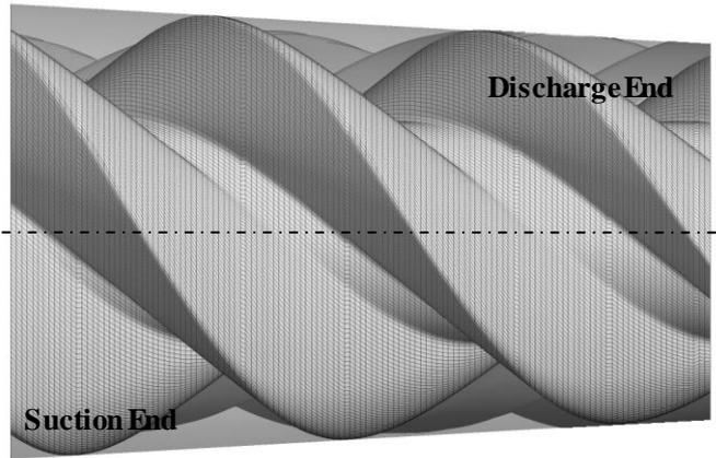
**Figure 7. Numerical grid for uniform pitch, variable profile rotors**
