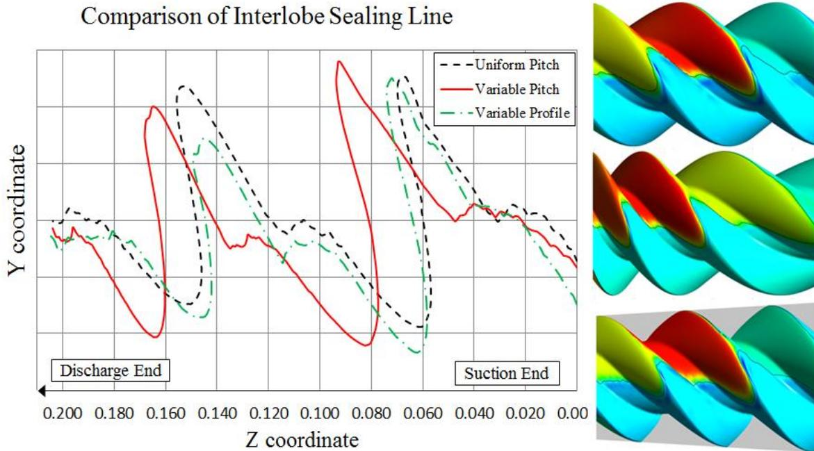
**Figure 12. Comparison of interlobe sealing line lengths**
